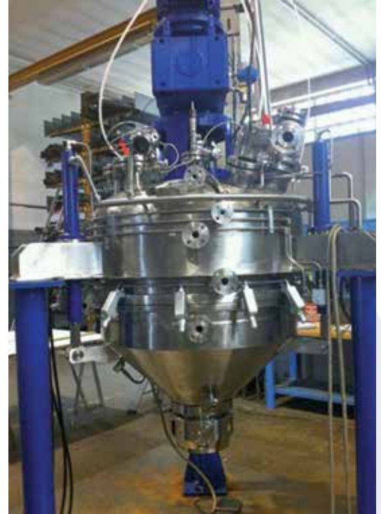
Condry ® conical bottom agitated vacuum dryer, left in Titanium Grade 7, right in Hastelloy C 22.
