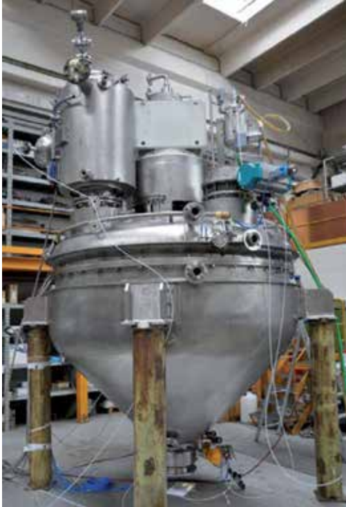
Condry ® conical bottom agitated vacuum dryer, left in Titanium Grade 7, right in Hastelloy C 22.
