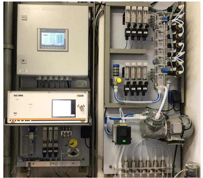
Figure 5: GC-IMS on-site integrated into process measuring and control technology system of Bilfinger Maintenance GmbH.
