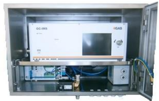
Figure 6: GC-IMS instrument for monitoring of TICs in chemical plants embedded into a pressurized enclosure system. The pressurized enclosure system ensures safety class Ex II 2 G Ex px II T4 (German Explosion Protection Ordinance).
